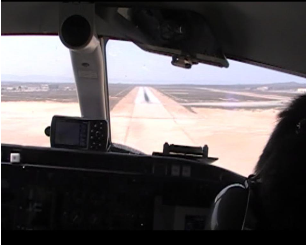
Figure 4: Learjet Surrogate UAV Flown Remotely to Landing with a Two Second Datalink Delay
