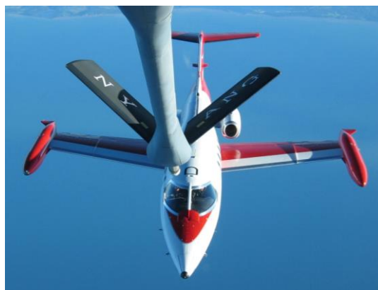
Figure 1: Learjet Surrogate Flying Autonomous Formation with KC-135
